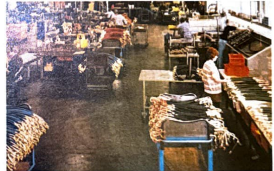
Pressure testing of production hose assemblies and fittings at Baden-Baden. ▽
