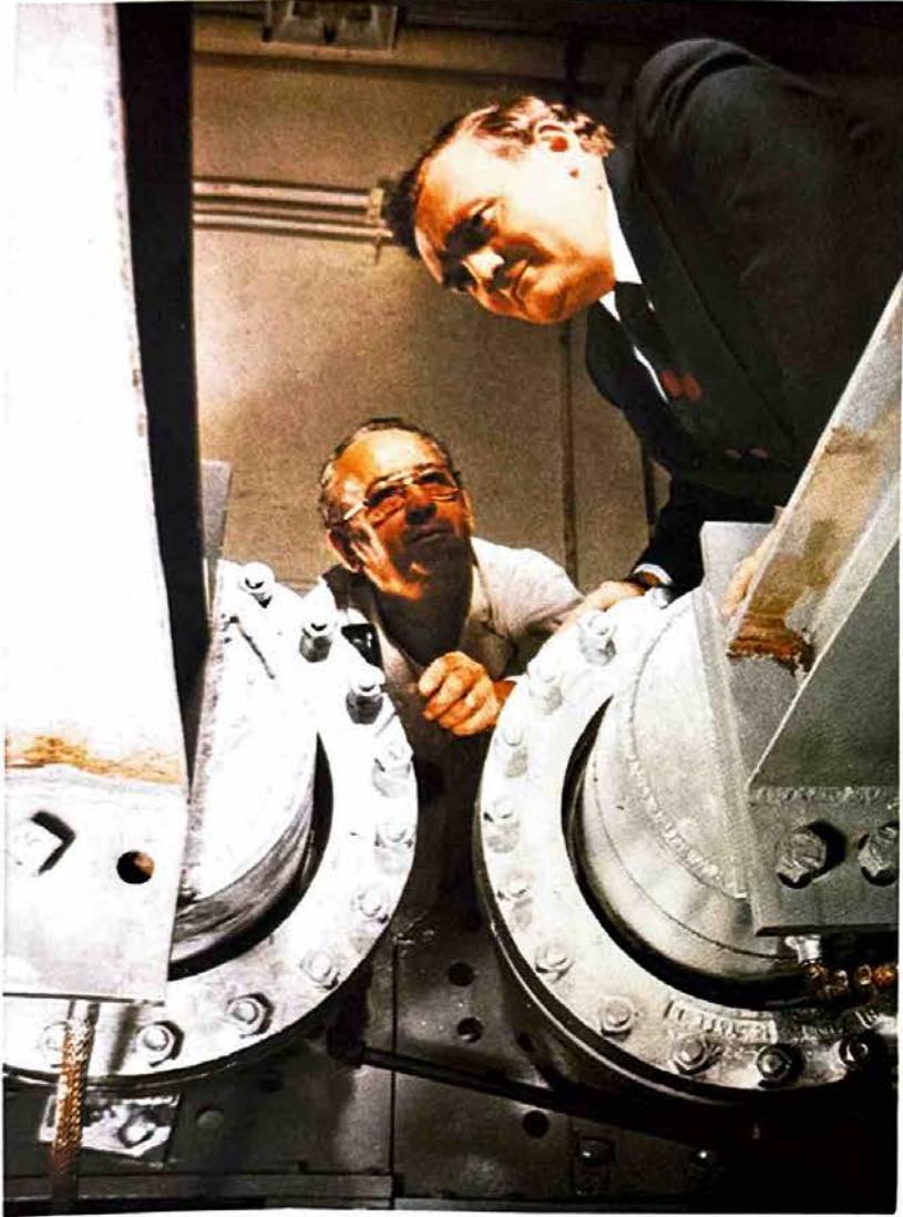
△ Barco Ball joints in the final stages of preparation for high temperature testing.
