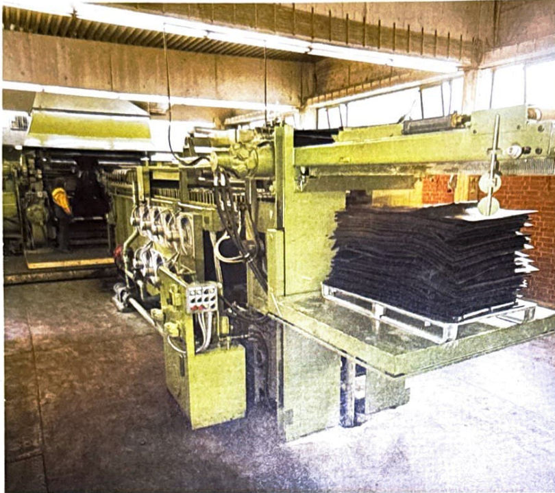
△ At Hann. Muenden, batches of rubber pass through this specialised cooler after milling.
