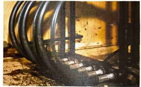
Aeroquip swaged hose assembly undergoing cycle impulse testing. ▽
