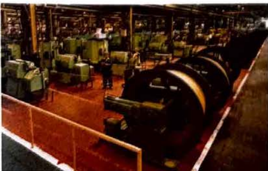
◁ A bank of high speed braiding machines manufacturing long length hose on flexible mandrels at Cardiff Works. ▷
