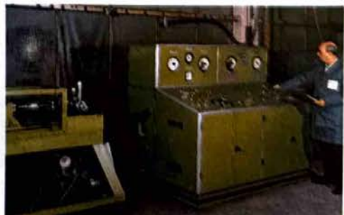
Testing of flexmaster joint for pressure, impulse pressure, temperature rating and vibration resistance under axial and radial loads - Hann. Muenden, West Germany.
