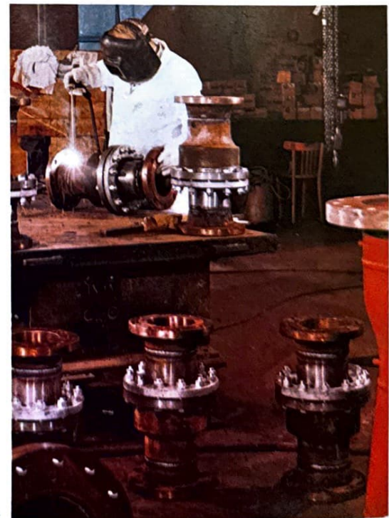
Pipe flanges being welded to Barco Ball joints at the Yates- Barco Works, Marple, Cheshire. ▷
