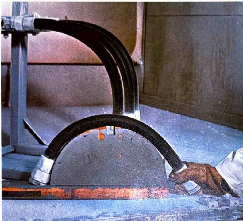
◁ Corporate Laboratories carry out wide ranging tests on all Aeroquip products. Pictured left is AQP hose undergoing bend radii testing under extreme low temperature conditions.
