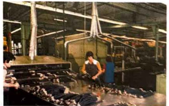
At Baden-Baden product is pictured undergoing cleaning and capping before final inspection and despatch to customer. ▷
