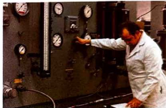
Flow testing a self-sealing quick disconnect coupling.
