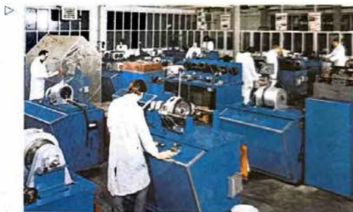
Seals undergoing simulated operating conditions on specialised laboratory rig testing equipment at Cardiff Works.
