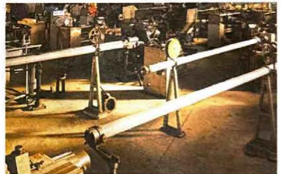
Hose fittings undergoing final stages of manufacture on single spindle machines at the Aeroquip Livorno plant in Italy. ▷
