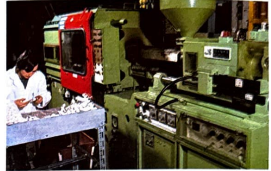
△ Automatic, gravity fed plastic injection moulding machines provide quality and consistency at Plastics Division, Kings Norton, Birmingham.
