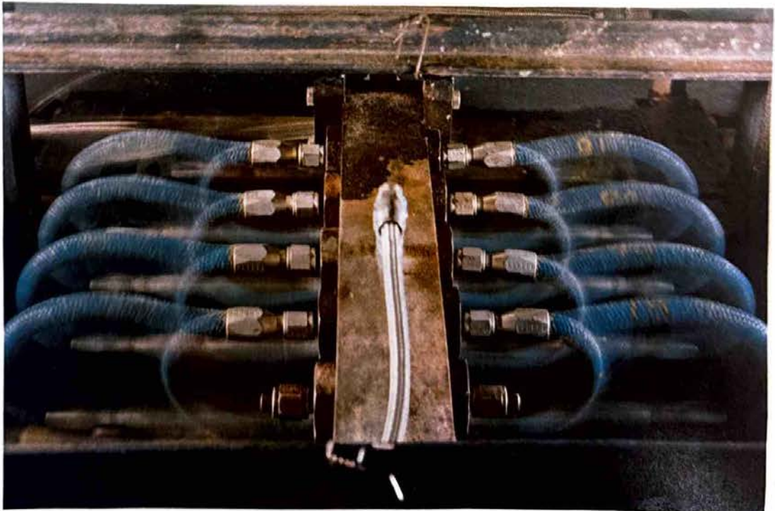
FC300 AQP hose undergoing continuous flex cycle and temperature testing. ▷
