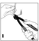
Brake Tube Pliers allows a tight 90° bend on the brake tube, right at the tube nut.
